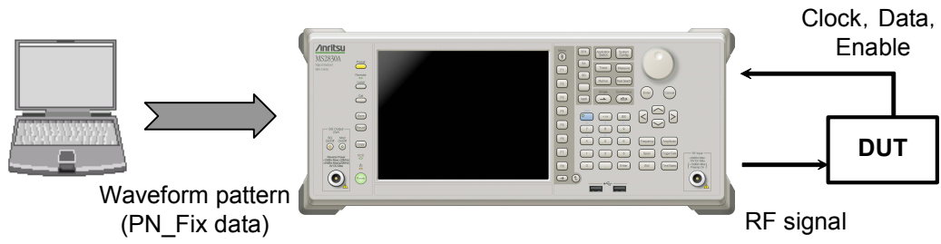
Figure 8.8-6 BER measurement using PN_Fix data
